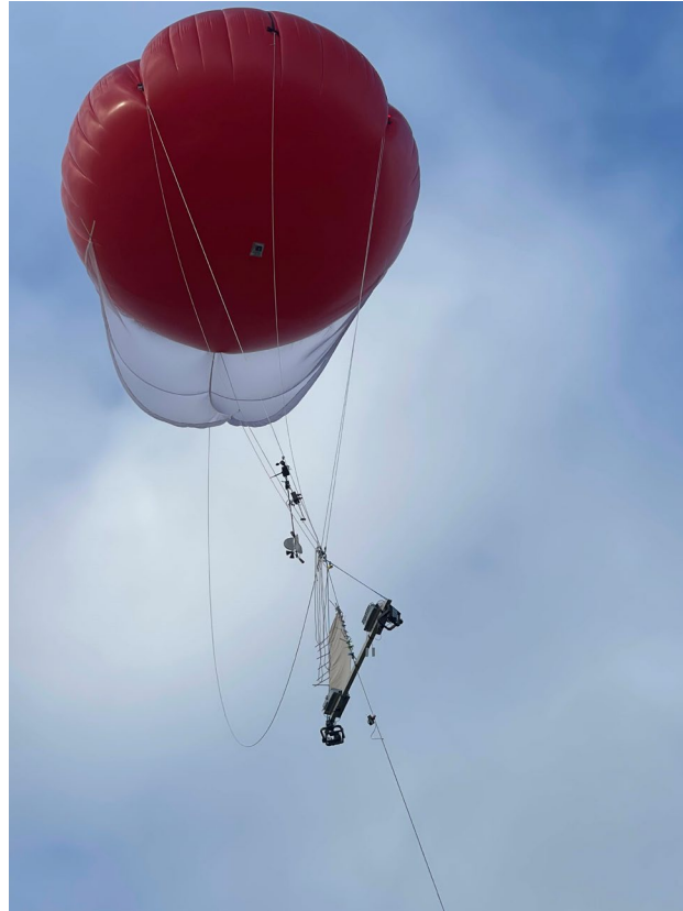
Tethered Balloon System (TBS): partnership with Sandia NL to monitor wildlife interactions with ME devices using a diverse optical and thermal payload
