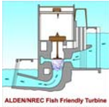
ALDEN/REC Fish Friendly Turbine
