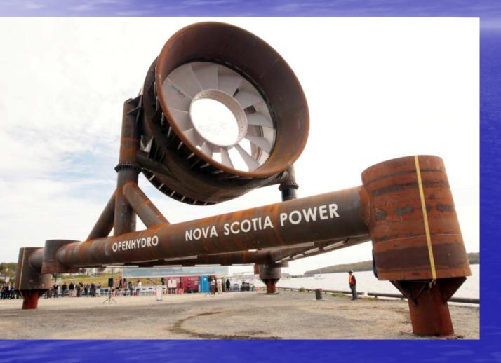
Admiralty Inlet Project proposes the temporary installation of two 10-meter, grid connected OpenHydro turbines.
