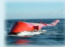
Attenuator (Pelamis) Source: Pelamis Wave Power
